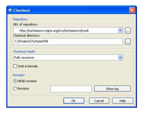
Figure 5.7. The Checkout dialog
