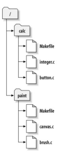
Figure 2.6. The Repository's Filesystem
