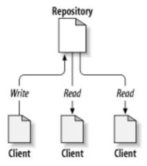
Figure 2.1. A Typical Client/Server System
